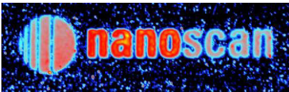
Non-contact AFM topography image of the NanoScan logo patterned by ion-sputtering on a Cu/Al/Si multilayer sample. Image size is 32 \times 10 \mu\text{m}^2 .
