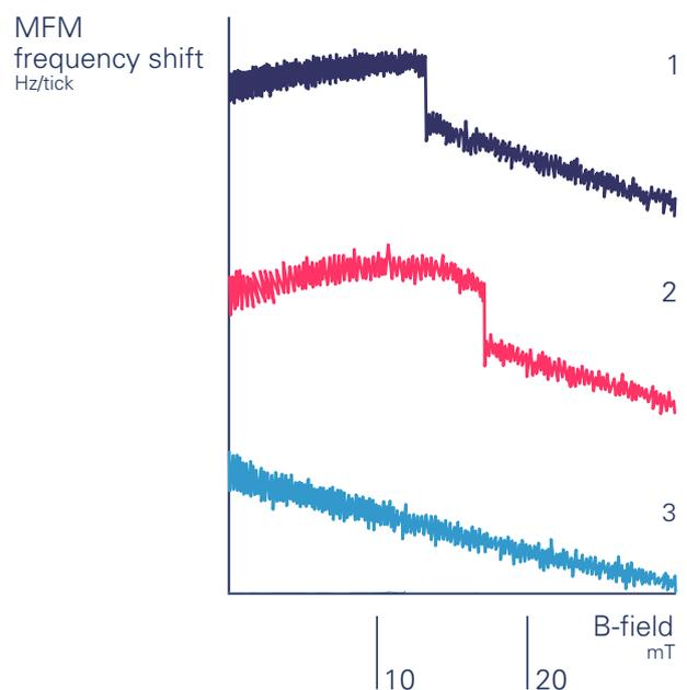
Trace 1 shows a core flip in a positive field of 13 mT. Trace 2 shows the core flip at negative field of -17 mT. The last sweep (trace 3) shows only linear decrease of the signal without any abrupt changes as the vortex core was already flipped in the previous sweep.
