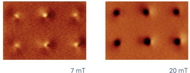
The frequency shift of the MFM cantilever positioned above the centre of a single cobalt nanosphere with a radius of 150 nm is measured during a magnetic field sweep.
